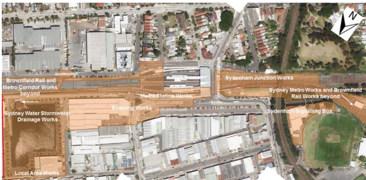
Figure 3: Sydenham Metro upgrade scope of work
