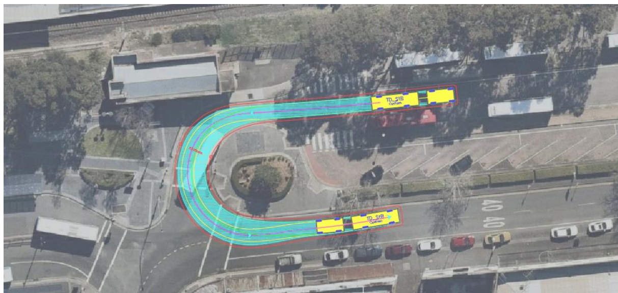
Figure 13 – Satellite Compound: Left-turn Exit
