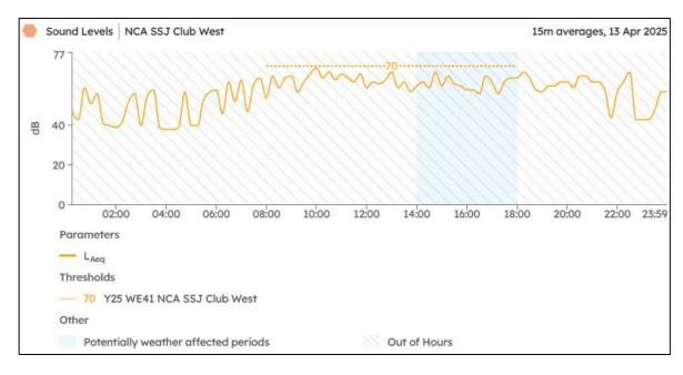
Noise monitor detect highest LAeq15min value at 74dB above the prediction (73dB), between 1015 to 1030.
