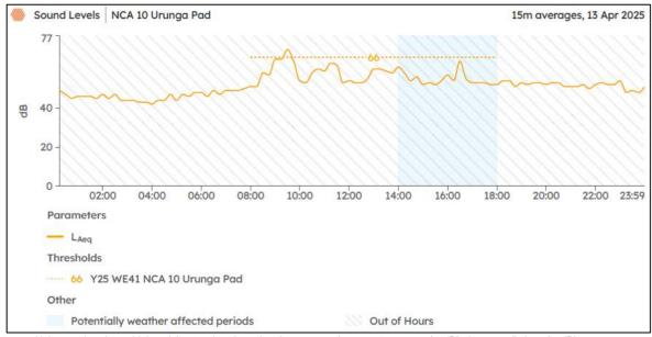
Noise monitor detect highest LAeq15min value related to construction at 0915 to 0930 (70dB) above predictions (66dB). Predicted noise levels (Dayshift works) in this area did not trigger offers for additional mitigation measures. Actual noise levels (Dayshift works) in this area did not trigger offers above the Respite limit. Appropriate mitigation measures being offered. No further additional mitigation measures required.
