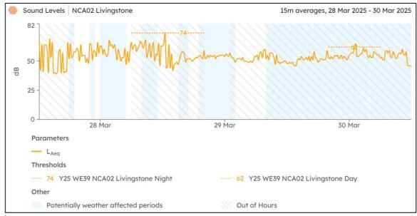
ARTC De-Vegetation adjacent to Monitoring point identified between 1300-1315. Laeq for time period 1300-1315 recorded at 65 dB, above the prediction (Laeq=62 dB). Data for time period 1300-1315 not related to JHLOR activity.
