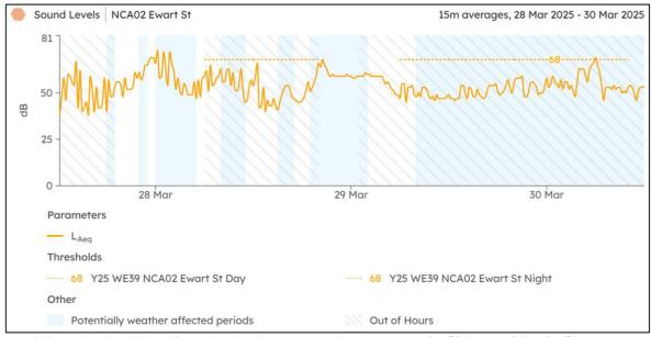
Noise monitor detect highest LAeq15min value related to construction at 1745 to 1800 (69dB) above predictions (68dB). Predicted noise levels (Dayshift works) in this area triggered offers for additional mitigation measures. Actual noise levels (Dayshift works) in this area did not trigger offers above the Respite limit. Appropriate mitigation measures being offered. No further additional mitigation measures required.
