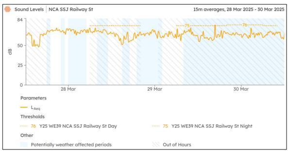
Noise monitor detect highest LAeq15min value related to construction at 0400 to 0415 (76dB) above predictions (75dB). Predicted noise levels (Night shift works) in this area triggered offers for additional mitigation measures. Actual noise levels (Night shift works) in this area did not trigger offers above the Respite limit. Appropriate mitigation measures being offered. No further additional mitigation measures required.
