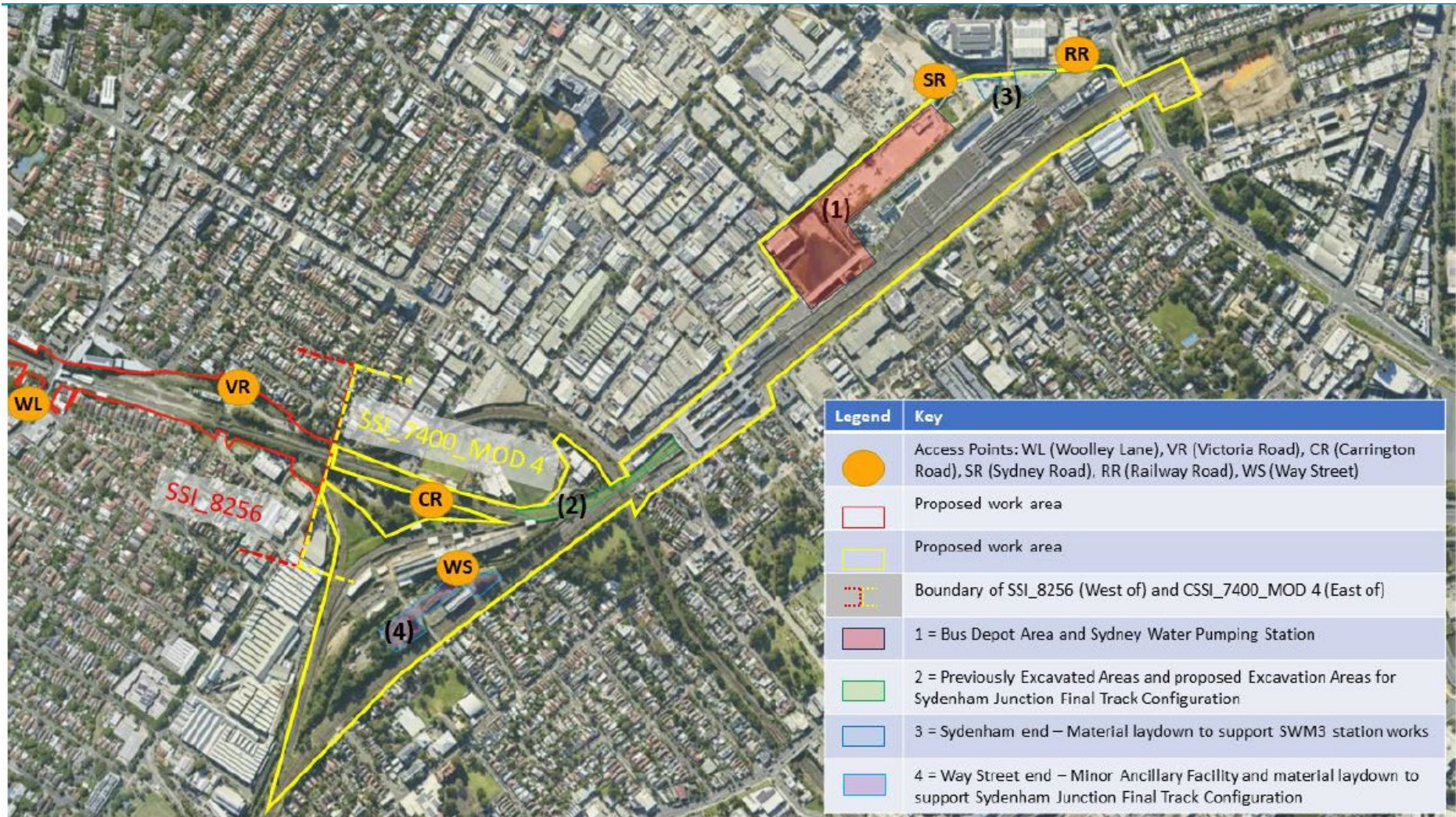
Figure 1 Sydney Metro Marrickville to Sydenham Site Layout (source: Sydney Metro City & Southwest - Sydenham to Bankstown -Planning Approval Consistency Assessment Form: Final track configuration works to complete the connection between Marrickville Station and Sydenham Station, October 2023.)
